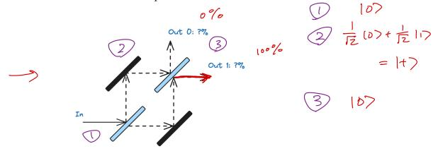
It turns out that the beam splitter acts like a Hadamard gate, and the horizontal "input" is like a  $|0\rangle$  state, and the vertical "input" is like a  $|1\rangle$  state.  $\times$
