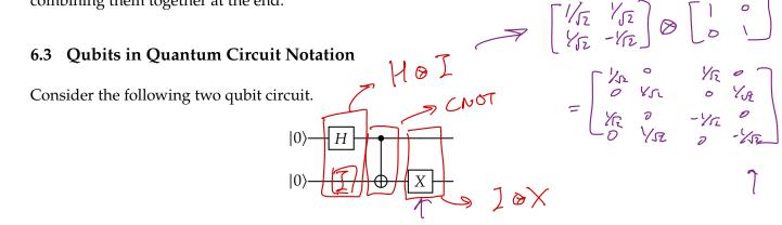
The circuit starts in the state  $|00\rangle$ . We then apply an *H* gate to just the first qubit, and then a CNOT gate with the first qubit as the control (a black circle represents the control bit).
